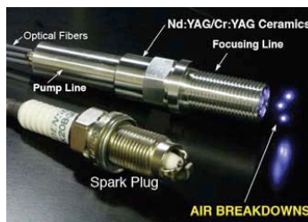
Fig. 1. Photograph of a laser igniter and current spark plug. This figure was already published and therefore its reference should be shown clearly [1]. The format of the reference is explained in the 5 th section in this style-guide.
